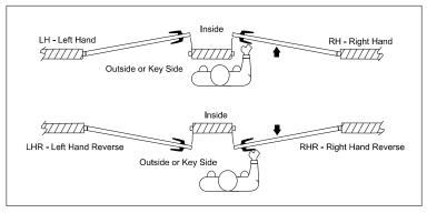
LHR/RHR is not necessary to specify for trim; it refers to the latch direction, which is not set on the Multipoint lock cases. INOX only provides the trim.
